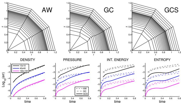
Figure 7: *Coggeshall test (adiabatic compression) calculated by an area-weighted scheme, the volume consistent but non-symmetric GC scheme [62], and the symmetrized scheme GCS [91]. Top: computational mesh, bottom: evolution of logarithm of  $L_1$  error in time*
