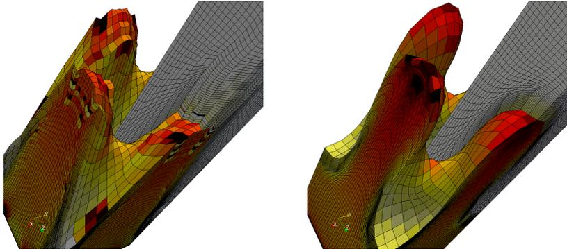
Figure 5: *Simulation of a hydrodynamic instability using classical edge artificial viscosity (left) and the new method [61] based on cell-centered Riemann solver (right)*
