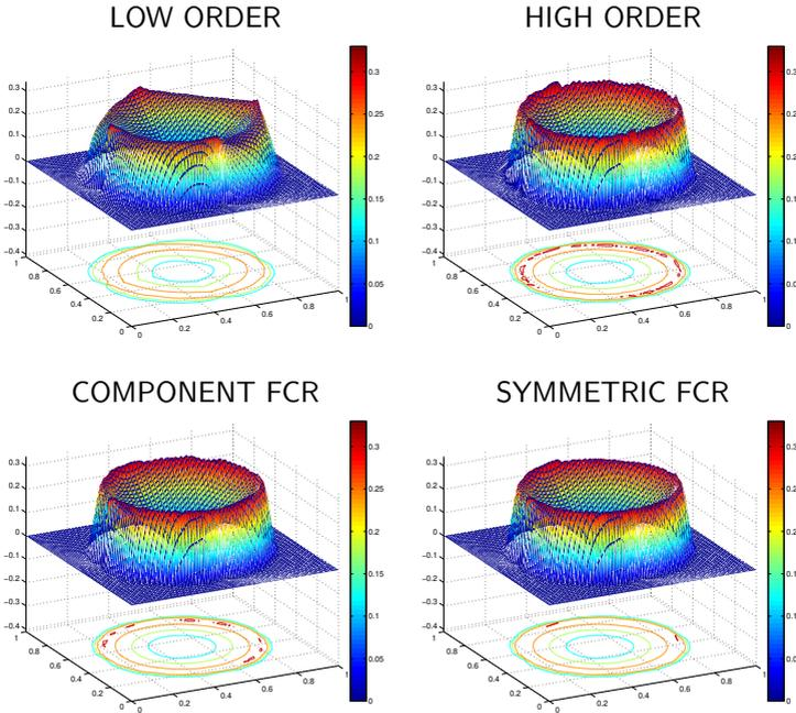
Figure 11: *Velocity magnitude for a point-symmetric problem with cyclic remapping on a logically rectangular mesh. Low-order remap (top left), unlimited high-order remap (top right), component-wise FCR in coordinate directions (bottom left) and symmetric FCR (bottom right) [94]*
