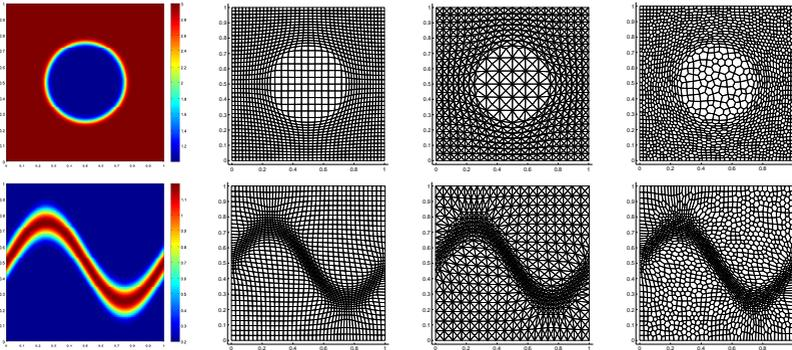
Figure 9: *Adaptation of various meshes to an underlying function by weighted condition number smoothing* [88]
