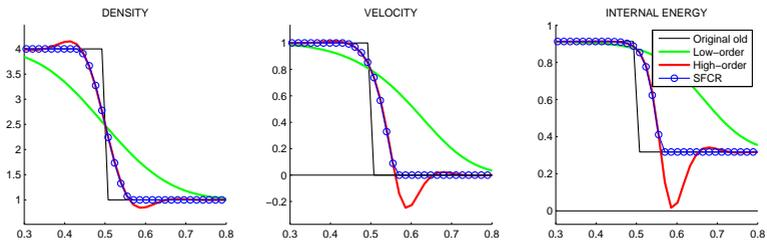
Figure 10: *The principle of flux-corrected remapping (FCR): use as much of high-order fluxes as possible while preventing overshoots and undershoots (preserving local bounds) by falling back toward low-order fluxes where necessary [56]*
