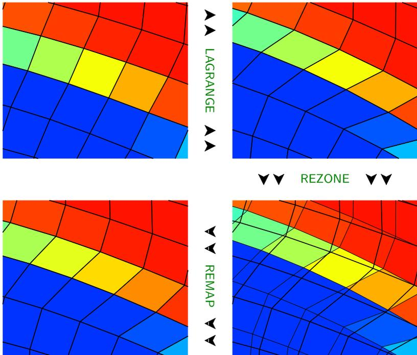
Figure 2: *Stages of the indirect ALE algorithm. Clockwise from top left: Lagrange step (advance in time), rezoning (mesh adaptation), remapping (transfer of solution onto the rezoned mesh)*
