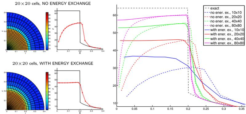
Figure 4: *Wall heating can be avoided or reduced by addition of a simple energy exchange term* [92]
