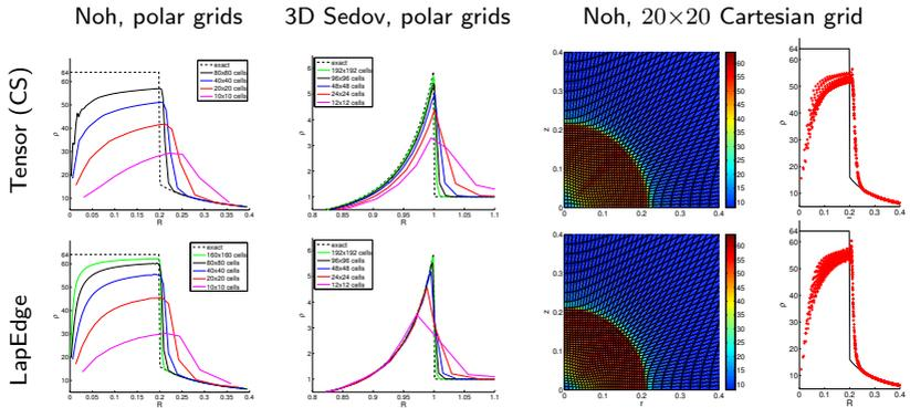
Figure 6: Comparison of area-weighted Campbell-Shashkov tensor artificial viscosity [11] (upper row) to the new genuinely  $r$ - $z$  approach LapEdge [90] (lower row)
