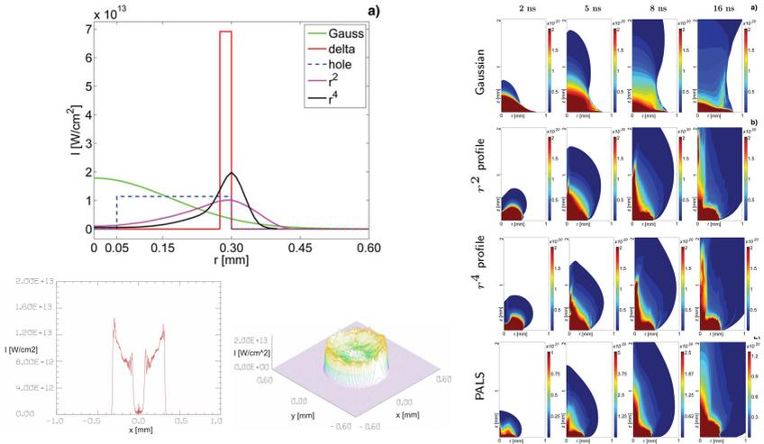
Figure 12: *Generation of collimated plasma jet outflows by annular laser beams. Left panel: Various radial intensity distributions of beams given by analytical functions (top) and calculated from a real experiment at PALS (bottom). Right panel: Evolution of electron density for selected beam profiles [42]*
