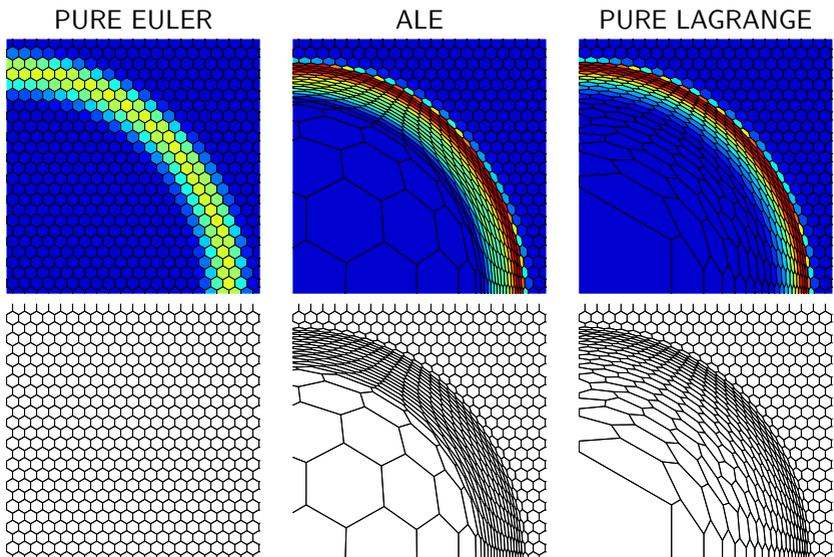
Figure 1: *Simulation of a point-symmetric shock wave (centered at the lower left corner of the plots) on an initially regular honeycomb mesh. Left: pure Eulerian calculation; right: pure Lagrangian calculation; center: Arbitrary Lagrangian-Eulerian (ALE) calculation*
