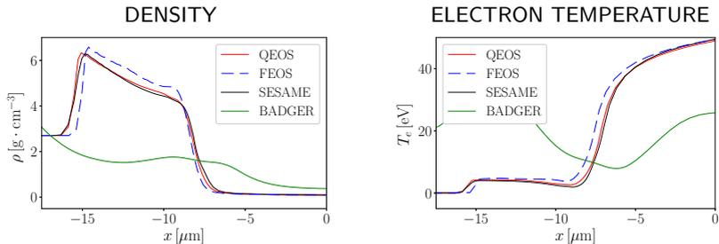
Figure 13: *Simulation of a laser pre-pulse. Profiles of density and electron temperature obtained with various EoS applied and compared using the HerEOS tool [101]*
