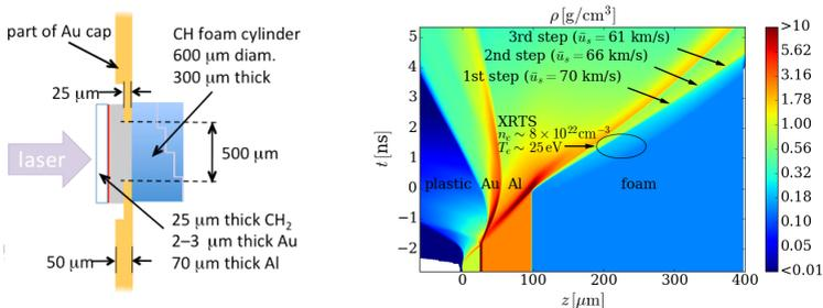
Figure 14: *Velocity of laser-driven shock in  $C_8H_8$  foam at OMEGA laser facility. Left: schematic picture of the multi-layer target. Right: result of the PETE simulation using SESAME EoS interpolated by HerEOS [101]*
