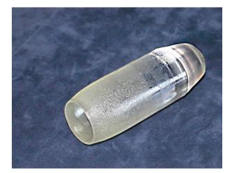
Figure 9 Photo of the Zr-codoped YAP:Ce single crystal (45 mm in diameter and 125 mm in length). Courtesy of the CRYTUR company.
