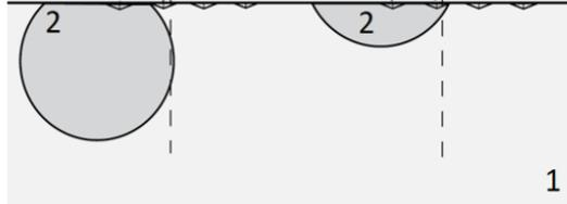
Fig. 3 Schematic illustration of indentation in proximity of the interface hidden below the indenter contact area.
